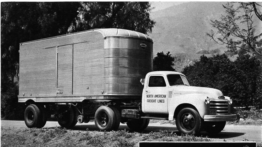
MODEL 6103 CHASSIS AND CAB 137-INCH WHEELBASE, MAXIMUM G.V.W. 16,000 LB.
