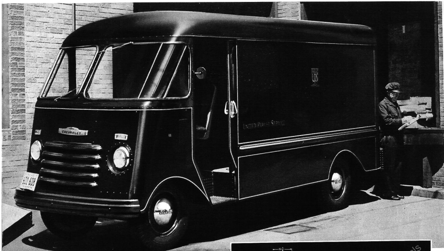
MODEL 3942 DUBL-DUTI 137-INCH WHEELBASE, MAXIMUM G.V.W. 10,000 LB.
