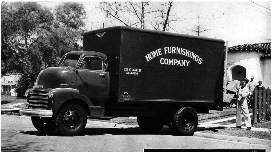
MODEL 5703 CHASSIS AND CAB 158-INCH WHEELBASE, MAXIMUM G.V.W. 16,000 LB.
