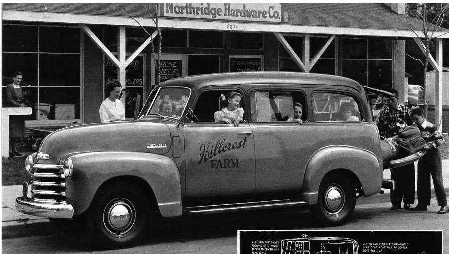
MODEL 3116 CARRYALL SUBURBAN 116-INCH WHEELBASE, MAXIMUM G.V.W. 4500 LB.
