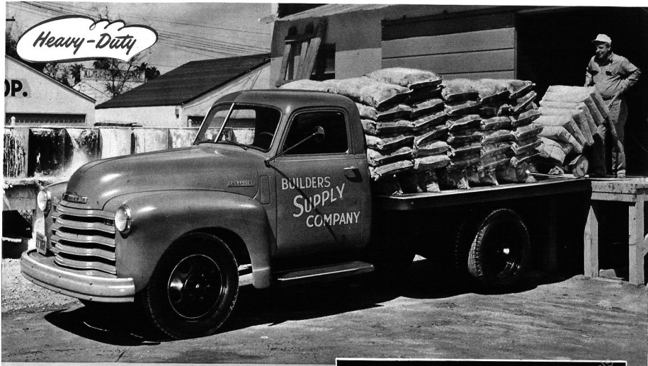
MODEL 4108 PLATFORM 137-INCH WHEELBASE, MAXIMUM G.V.W. 12,500 LB.
