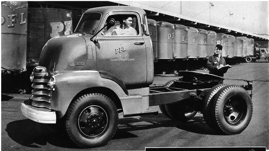
MODEL 5103 CHASSIS AND CAB 110-INCH WHEELBASE, MAXIMUM G.V.W. 16,000 LB.
