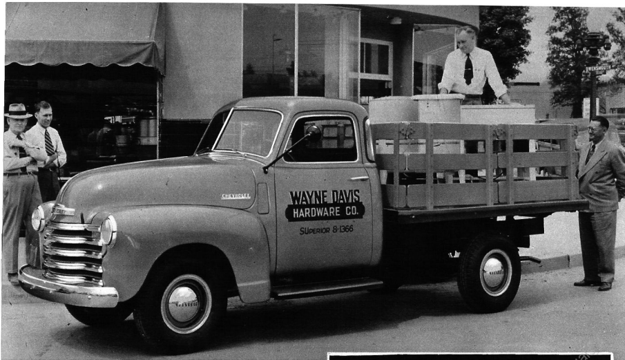
MODEL 3409 *DE LUXE STAKE 128 \frac{1}{2} -INCH WHEELBASE, MAXIMUM G.V.W. 5800 LB.
