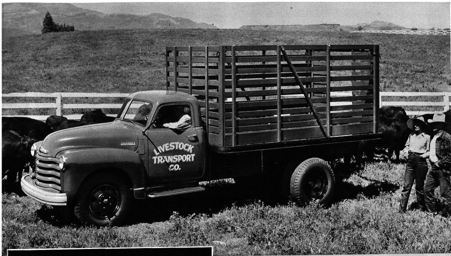
MODEL 6419 HIGH RACK 161-INCH WHEELBASE, MAXIMUM G.V.W. 16,000 LB.
