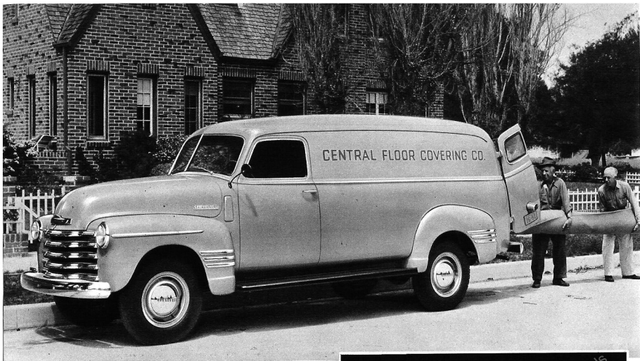
MODEL 3805 *DE LUXE PANEL 137-INCH WHEELBASE, MAXIMUM G.V.W. 6700 LB.
